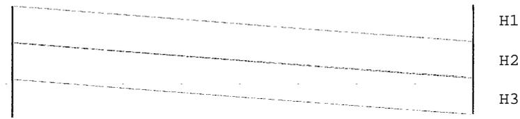
If a pattern or the oblique line contains gaps (see the examples on the next page), the contact areas and the cable contacts of the affected print head must be cleaned, or the affected print head must be replaced (see Section 9.4 -Notes on maintenance).
